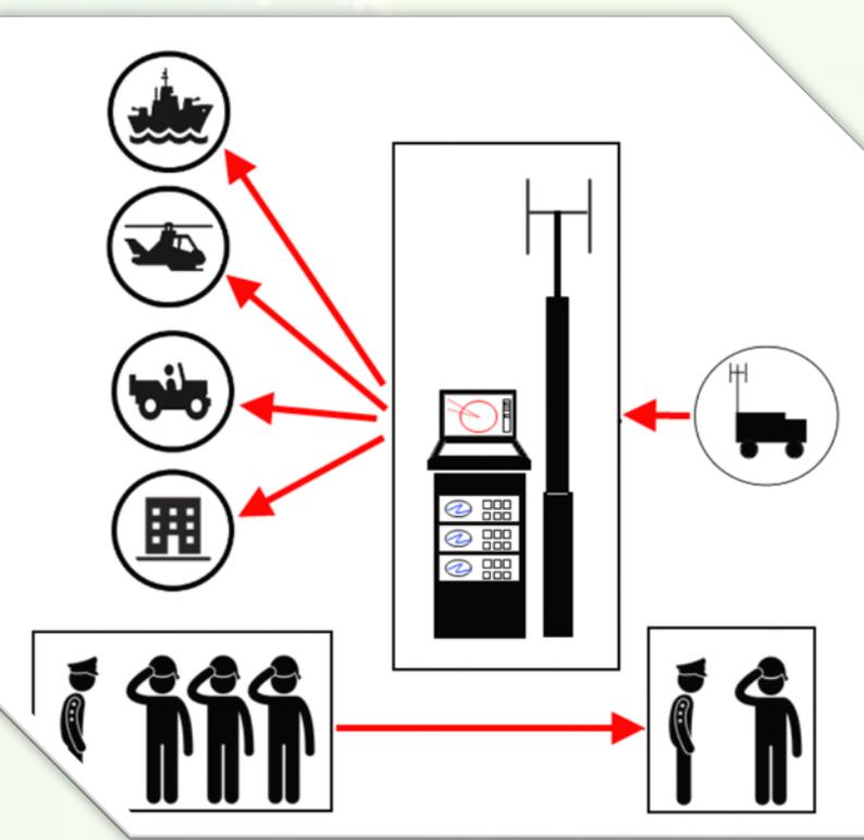
The ability to remotely control our radio surveillance network, allows to create networks of autonomous radio surveillance stations under a single control and configure the radio surveillance network according to the tactical situation and tasks. It allows reduces the number of qualified personnel for network maintenance.
