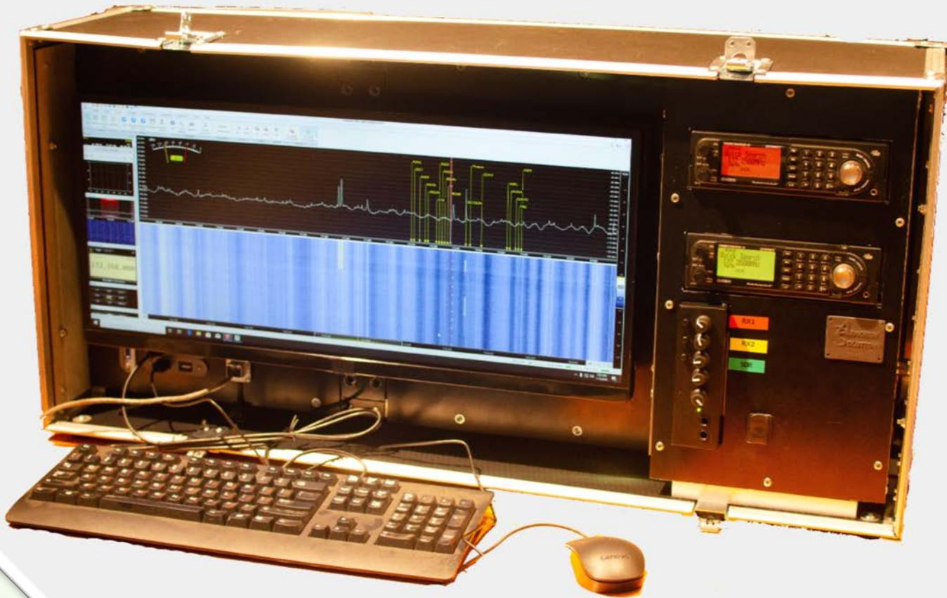
Modular SIGINT/COMINT Radio Surveillance System " Tin-MD "in the form factor of an autonomous portable container.
